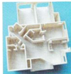
The three-dimensional foam models of facilities can show both the exterior and interior of buildings.
