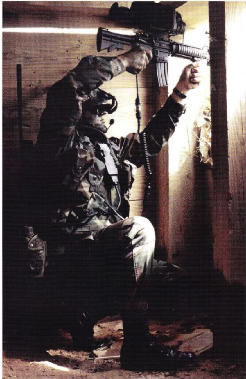
A soldier uses a gun-mounted camera with an eyepiece to obtain a remote look into an area he is about to enter. Technology advancements like this one are driving the Analysis and Plans Office's ongoing future needs assessments.
