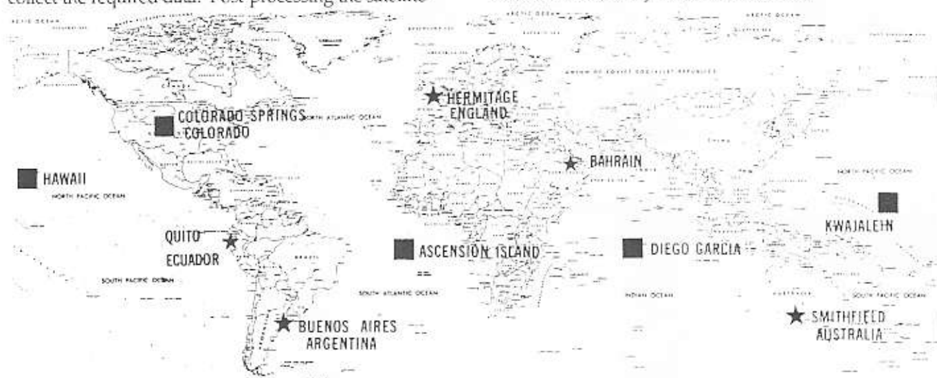
This map shows the disposition of GPS earth stations. The DMA GPS tracking network is identified with stars; the squares are monitor stations of the Air Force's Operational Control Segment (OCS), from which additional data is received.
