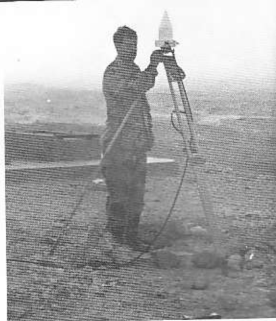
Sergeant Pete Patera uses an antenna placed on a tripod to collect survey data in Saudi Arabia during Operation Desert Shield.
