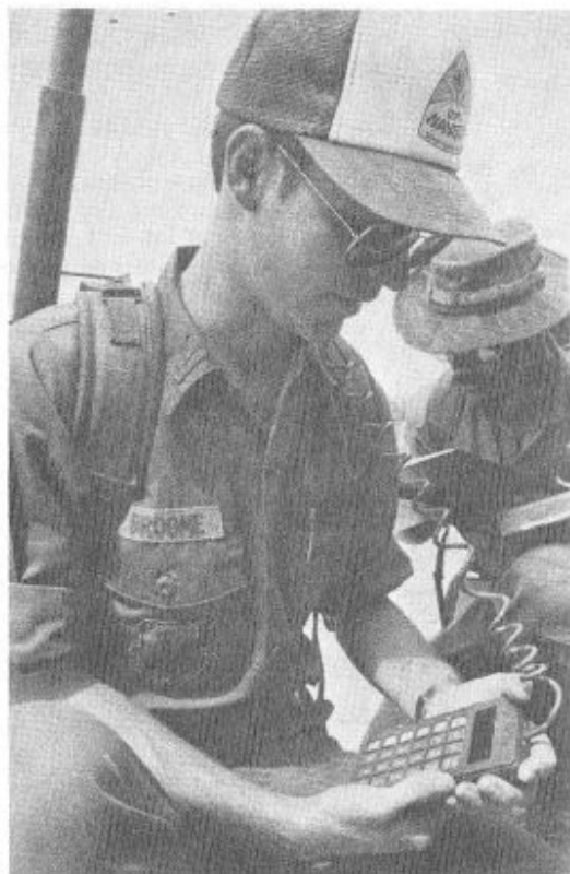
First Lt. Lynn Broome of Edwards AFB, Calif., uses the Navstar manpack receiver to determine his location during tests at Yuma Proving Grounds, Ariz.
