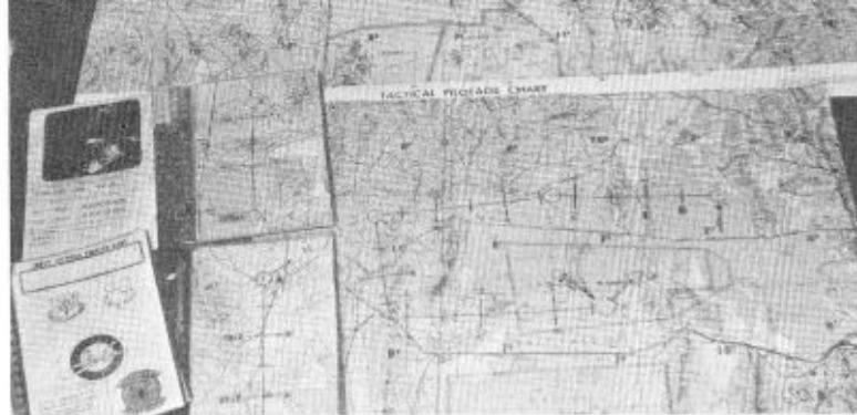
Pilot booklets assembled by the intelligence section are compiled from Tactical Pilotage Charts on which specialists draw routes to the ranges and post navigational aids on selected chart portions. Pilots carry the booklets on their flights for quick and easy reference. (U.S. Air Force Photo by SSgt. Denise E. Cornella, 388th Tactical Fighter Wing, Hill AFB, Utah)
