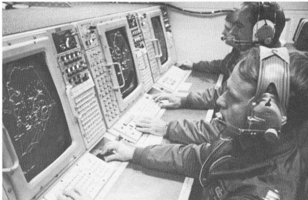
Data supplied by the Defense Mapping Agency is used to create those computer-generated map displays on the multi-purpose consoles of mission crew members flying on the Airborne Warning and Control System aircraft. [U.S. Air Force photo]
