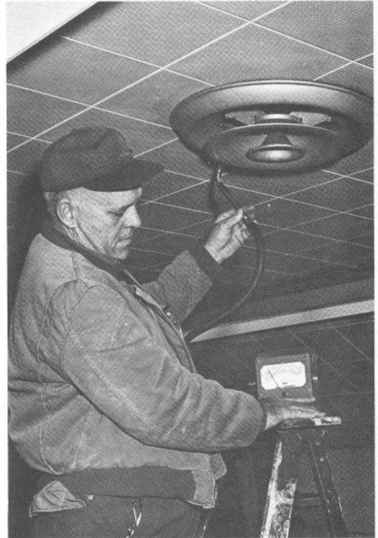
To make sure the heat comes through, Dean Evans verifies air velocity at a heating/cooling diffuser.
