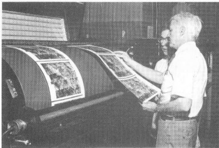
As the Skylab photo prints come off the auto-processor, they are checked by Raymond Roach, Quality Control Inspector and Warren Tabachik, section supervisor. Color control and exact representation were critical to the program.
