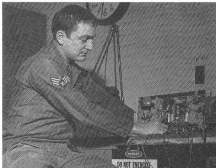
Sgt. Charles C. Alford makes a voltage check on a public address system amplifier.
