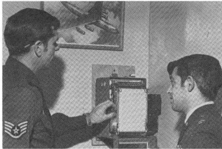
A printout on a telephone traffic usage recorder is explained to Capt. Salvatore Bosco, (right) commander of Det. 1, by SSgt. Robert J. Harris. The device measures the frequency and length of telephone calls at DMAAC.
